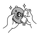
Clean the disc with water diluted with neutral detergent solution and wipe from inside to outside using dry cloth.
